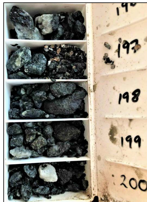
Figure 1: RC chips of sulphide and quartz-rich mafic rocks from hole 20SLGR17
