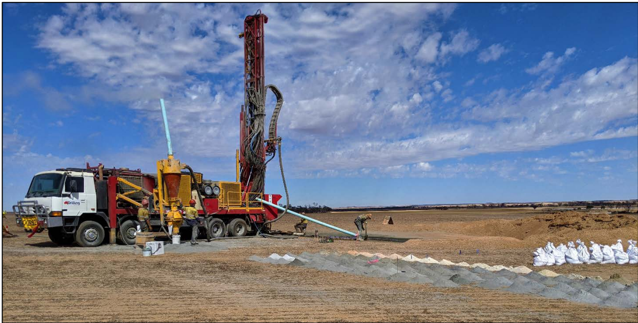
Figure 3: RC drilling at the Challenger Prospect, Lake Grace
